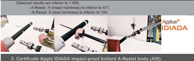
Obtained results show a level of acceleration of the body which relates with a possibility of suffering from a damage of 12% gravity AIS3 for the model H.
