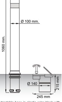
Extractable base in plastic color black with a float superior extremity. It has a standard triangular key located at the lateral side of the base so as to block the extremity when enclosed or to block the bollard when introduced in the hole.
