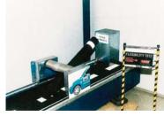
More than 6,000 bending cycles were performed without any slits appearing on the bollard surface and during which the bollard was returned to its original position after the force required to bend it to 90° was applied
